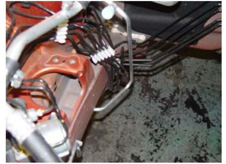
3. By removing the plastic anchor clips and gently bending the brake lines they can be moved to the area above the frame rail and allow for clearance with the K-series engine.
