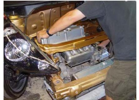
3. Once the car has been lowered and the engine is within a few inches of where the mounts are, install the left-hand transmission bracket using the Hasport hardware. You will place a spacer under the bracket on the outside rear mount hole so the bracket mounts flush. Leave the bolts finger tight at this time. Continue to lower the car until you can bolt the transmission bracket to the mount. Use the stock bolt and Hasport supplied nylon lock nut.
