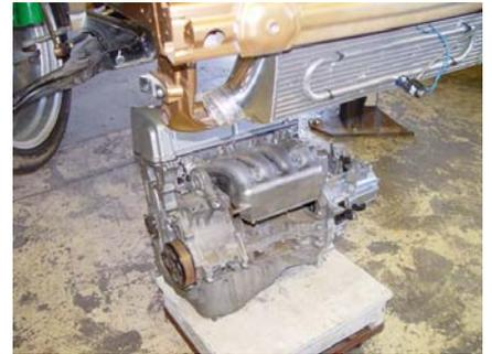
2. Lower the car slowly taking care not to hit the engine on the way down. Keep close watch on the VTEC solenoid on the rear of the engine and the clutch actuator fork and slave cylinder on the front of the transmission. You may need to twist the engine while lowering the car to avoid contact. This is a two-man job.
