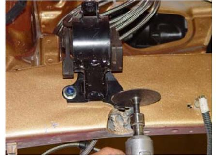
8. The core support sheet metal will need to be notched to clear the intake manifold. You will need to lower the car over the engine to see where the core support will interfere with the manifold. Make sure you have at least 1 inch of distance between the manifold and the core support sheet metal. This is necessary to prevent the intake manifold from coming into contact with the core support under acceleration.
