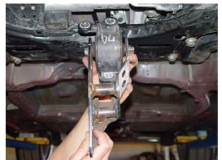
10. Next bolt the Hasport rear bracket to the engine and transmission. The front hole will use the stock bolt we removed in Step 10 while preparing the motor. The other two holes will use the Hasport provided hardware. Once all three bolts are in, torque to 47 lbf-ft. Torque the rear mount hardware to 43lbf-ft. Next torque the bolt holding the rear bracket to the rear mount to 51 lbf-ft.
