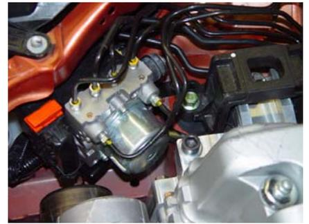
5. Brackets will have to be made to hold the ABS unit away from the engine. We opted to modify the stock bracket.
