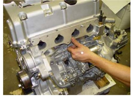
5. Cable operated throttle bodies should be removed from the manifold to prevent possible damage to the TPS or EICV while installing the motor.
