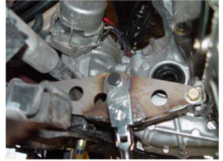
11. Install the K-series Fit swap axles and torque axles nuts to 134 lbf-ft
