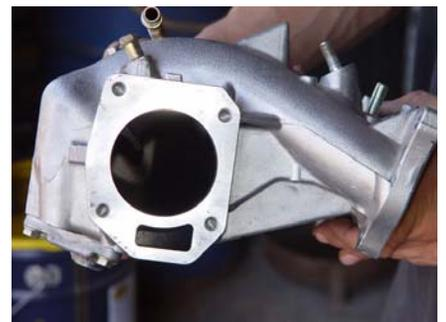
4. If your engine is one of the following engines, K24A2, K20Z3, or K24A4, you will need the Hasport Intake adapter to bolt the snail style manifold on. This adapter is to bypass coolant through the head while the thermostat is closed during warm up.
