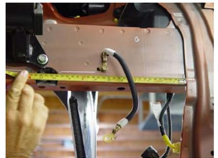
7. The engine mount will also need to be trimmed. Trim the metal that hangs down in to the opening you just made in the frame rail.
