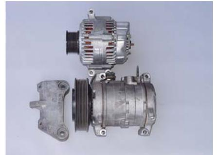
**WARNING: The snail style manifold will interfere with the alternators from the Accord, TSX and 06-07 Civic Si. An alternator from a 02-05 Civic, RSX or CR-V must be used.**
