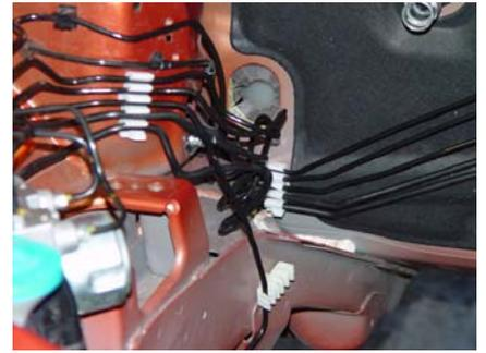
4. The ABS Modulator-control unit will also interfere with the K-series engine idler pulley and tension pulley. Tuck the ABS unit under the frame near the headlamp to clear the engine.
