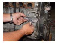
6. Bolt the EF alternator bracket to the adapter using the stock hardware. The oil dipstick tube will need to be bent slightly so it does not interfere with the alternator bracket.
