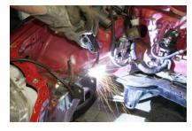
Clearance the chassis frame rail to make room for the transmission case. Use the sawzall and die grinder to cut a notch as wide as the right hand engine bracket under the frame rail bracket. Lower the car over the engine to get an idea where to cut the frame rail. Make sure you reinforce the frame rail after you have removed the material from the frame rail!
