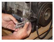
9. At this point you can install the EF alternator using the stock hardware. It will mount upside down as compared to how it mounted on the EF engine. You can also wait until the engine is in the vehicle.
