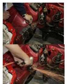
Bolt the bracket back onto the frame-rail. Stitch-weld the right-hand engine bracket to the passenger side frame rail.
