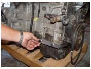
8. Bolt the EF alternator adjusting plate onto the bracket using the 10mm x 25mm bolt provided.
