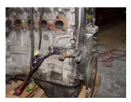
7. Bolt the alternator adjusting plate bracket to the block using the two 10mm x 45mm bolts.
