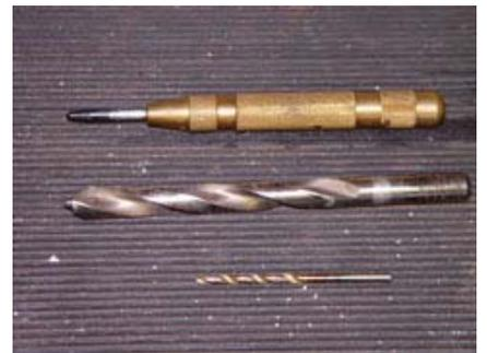
3. Begin by center punching all the spot welds on the mount. This is so the drill bit won't drift when drilling. Next use the 1/8 inch drill to drill a hole approximately 3/16 inches deep. This will prevent the pilot point drill from drifting. Don't worry if you drill completely through the sheet metal. Now use the pilot point drill to drill a hole as deep as the bracket sheetmetal is thick.
