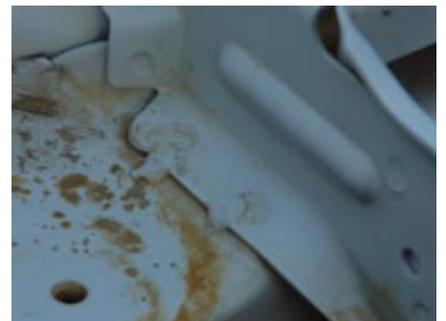
5. A chisel and hammer can now be used to finish removing the bracket. Once it is off use the die grinder with a sanding wheel to remove any excess material left over.
