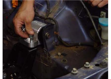
6. Bolt the right-hand mount to the engine bracket using the two 12mm x 40mm bolts with 12mm washers. Now bolt the mount into the bracket with the 12mm x 120mm bolt, two 12mm washers and 12mm nylon lock nut. Now you can go back and torque all three mount's bolts to 43 lbs-ft.
