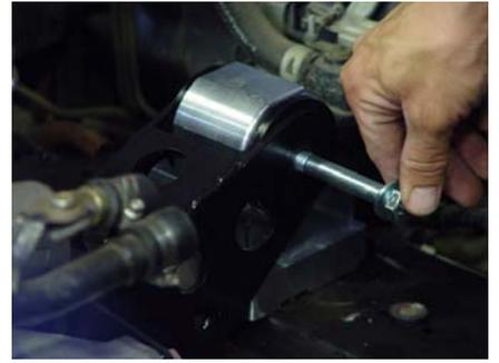
5. Connect the left-hand mount to the bracket using the two 12mm x 50mm hex bolts and 12mm nylon lock nuts. Use washers on top and bottom of the bolts. Tighten the bolts snugly.
