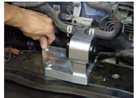
11. If you are installing the engine from the bottom, you can install the left-hand mount at this time. Use the original bolt for the Prelude mount for the new K-series mount.
